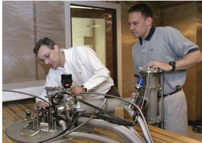
Dr. John DiTusa, LSU Professor of Physics and Astronomy, right, and Dr. David Young, Associate Professor of Physics, in an LSU lab with a refrigerator capable of cooling to hundredths of a degree above absolute zero.
