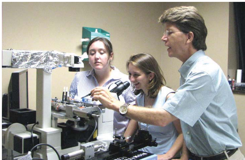
Tulane University graduate students Jerina Pillert, left, and Katharine Hamlington with Dr. Donald Gaver examine microfluidic experiments involving micro particle image velocimetry, an optical technique for measuring fluid velocity.
